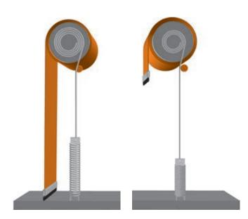
Tension springs are installed in the side frames and directly connected to the drive shaft by heavy load belts. The springs are taut in the position "Door is closed" (left) and slack in the position "Door is open".
