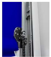
After the manual operation of the control, the door moves downwards into the closed position. All of the systems regenerate completely automatically: door curtain and closing edge are guided back to the frame by means of the tensioning ropes, the snap-in connections are connected again when the end position is reached.
