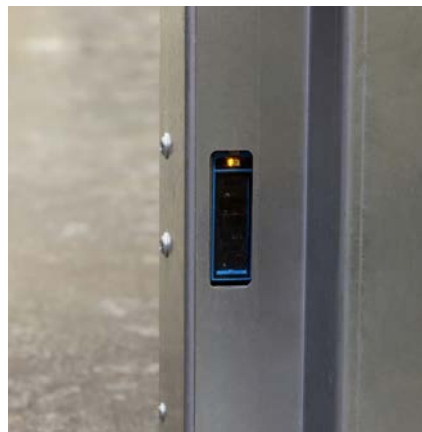
ATEX light barrier
